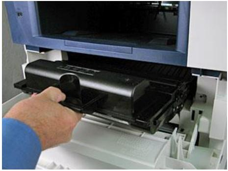
Open the front of the machine and remove the Smart Kit which includes everything that will need to be regularly changed. (Toner, Fuser, and Imaging Unit)
